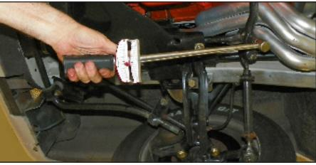
Making sure the top nut is very loose, torque the tapered stud nuts to 30 ft./lbs., and then keep tightening until a castle-nut slot aligns with the cotter pin hole. Install the pin.
