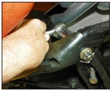
The top nut gets torqued last. This is actually the bearing preload adjustment. Dick will develop a torque value for this and supply jam nuts or prevailing-torque locknut. Now just slip the boot on, grease with MML, and adjust toe-in. Done!
