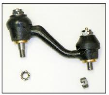
Firm Feel (www.firmfeel.com) has come to our rescue, with their Torrington-needlebearing equipped idler. It is not only greaseable, but adjustable. Even 50 years from now, simply snugging the adjuster nuts will reduce slop to zero.
